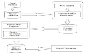
Fig 3. Architecture diagram of the proposed system
